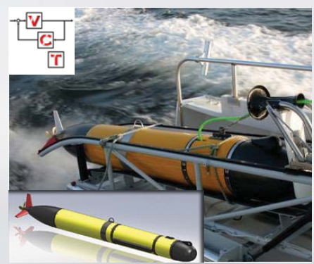
LMCS PTB - VCT's Powered Tow Body (UUV Convertible)
