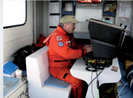
Operator views high resolution side scan sonar data in real time for quick identification of targets
