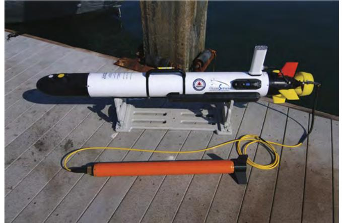
Fig. 1. IVER 2 AUV with EdgeTech 600/1600 kHz side-scan sonar, phase differencing bathymetry system, and an Explorer magnetometer.
