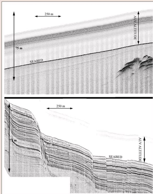
Figure 4. AUV subbottom profile comparison of typical seismic stratigraphy recorded in West Africa (top) and Gulf of Mexico (bottom).
