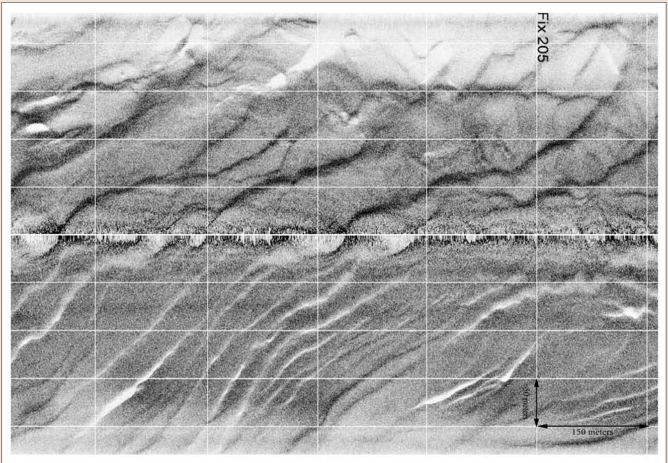
Figure 3. AUV side-scan sonar imagery (120 kHz) of intensely faulted seabed associated with near-seafloor salt in the Gulf of Mexico.
