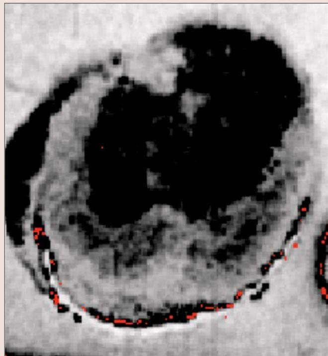
**Figure 7.** AUV microseismic (4 × 4 m bins) time slice through pockmark offshore Nigeria. Image measures 700 × 500 m (Data courtesy of Total).
