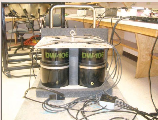
Figure 5. Subbottom profiler transducer upgrade (Edgetech DW106) undergoing lab testing. Increased source power levels and reduced beam widths should increase penetration depths to 150 m in clay-filled basins.
