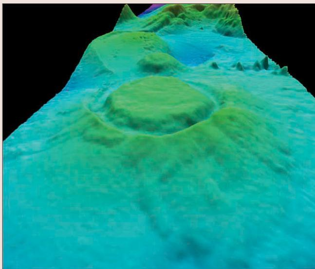
Figure 2. Fledermaus software 3D seafloor rendering of AUV bathymetry data (3-m bins) depicting a 220-m fluid expulsion feature found in the deepwater Gulf of Mexico (VE = 6x).
