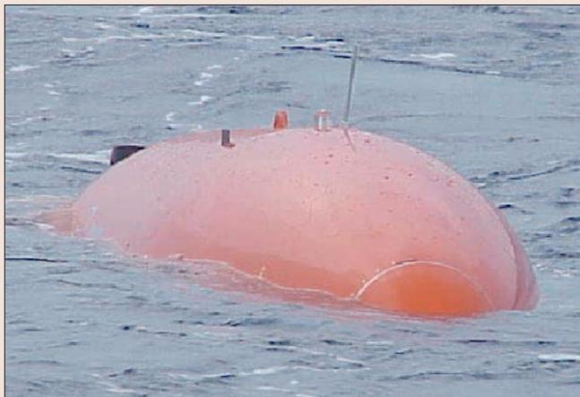
Figure 1. AUV going through the pre-dive system checks. System measures 6 m in length and 1 m in diameter.
