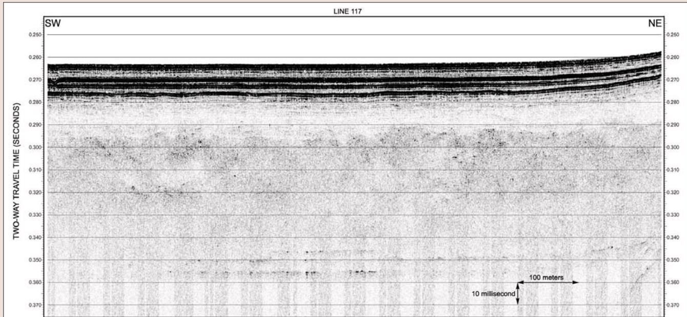
**Figure 6.** Subbottom profiler test data (1–6 kHz) collected from an AUV in a Norwegian fjord. The faint reflectors at more than 80 ms below the seabed provide favorable evidence for the desired increased depth of penetration.
