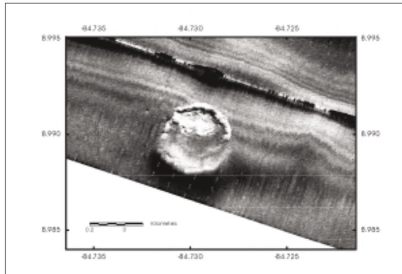
Figure 4: Part of 75kHz side-scan sonar profile from offshore Costa Rica showing a circular structure related to cold fluid seeps. Patches of high backscatter intensity (light tones) inside the crater are probably due to carbonate precipitation at the seafloor.
