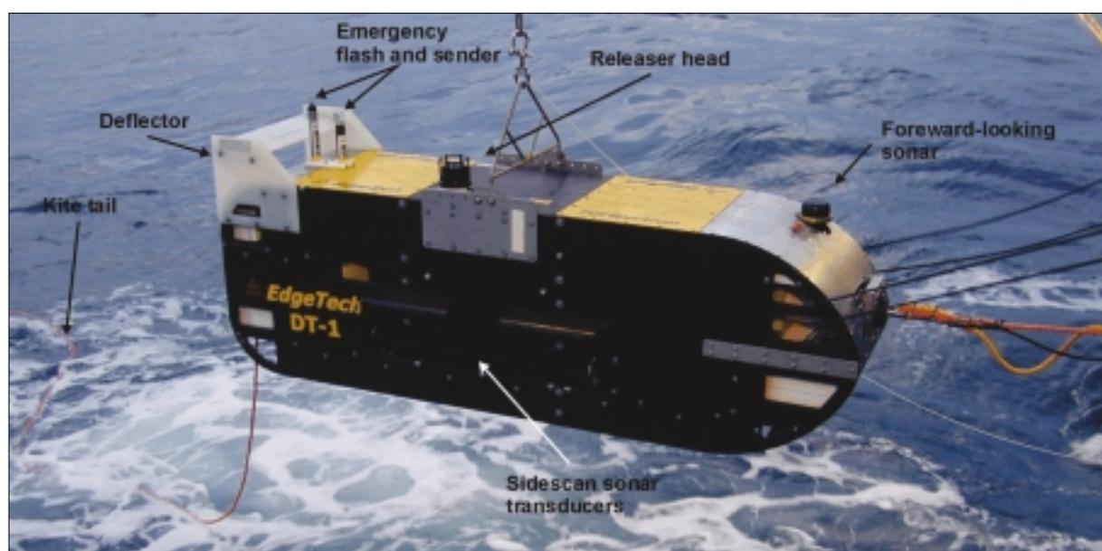
Figure 1: The DTS-1 side-scan sonar towfish during deployment.
