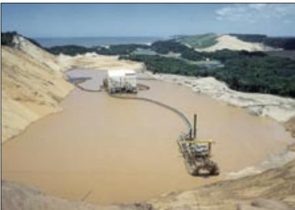
Figure 1: Mining dredger in rutile pit.
