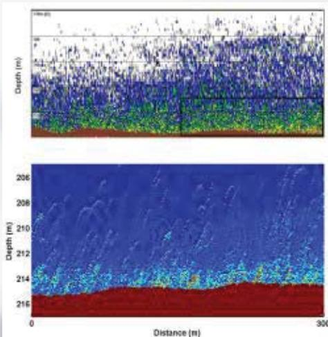
Top image from a narrow band acoustic system. Bottom image, showing fish, from the EdgeTech broadband system.
