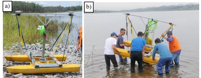
Fig. 3. a) catamaran float with sonar head, GPS antennae and motion sensor; b) catamaran being carried to the water.
