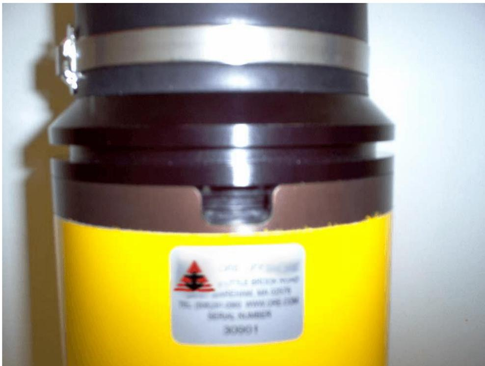
*Figure 3-2: Closure rod gland, rod removed*
