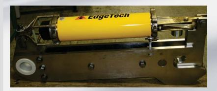
The HLR Heavy Load Release is a field-proven, reliable heavy duty acoustic release. The HLR strong back is made entirely of titanium to keep it light and strong. Titanium is also very corrosion resistant. We also use custom made Delran isolation washers to eliminate any risk of dissimilar metals causing corrosion. The HLR has been designed for easy use in both long term moorings and in lowering applications.
