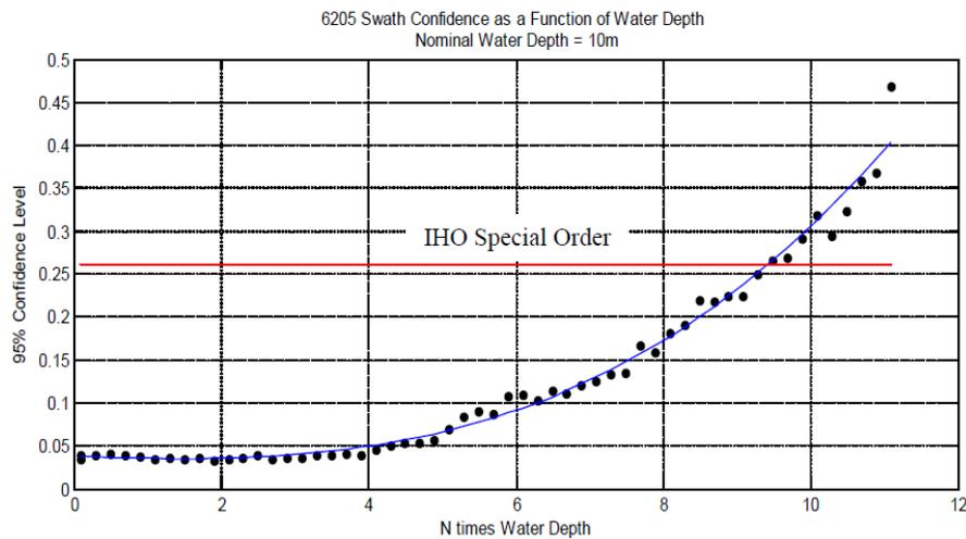
**Figure 1:** EdgeTech 6205 swath confidence as a function of water depth for a nominal water depth of 10m. IHO Special Order standard is indicated by the red line and equals 25.4cm for this particular water depth.
